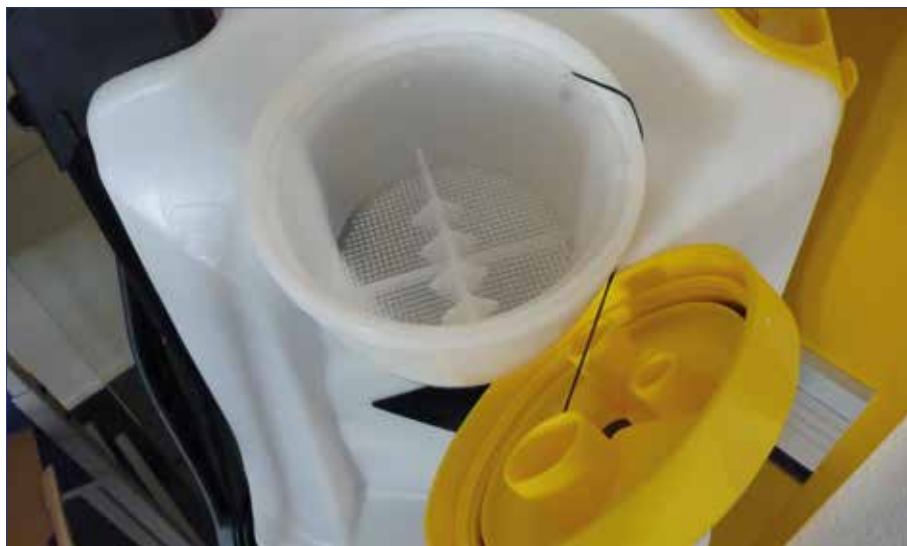
Figure 7. Equipment showing large opening and filter to facilitate filling
