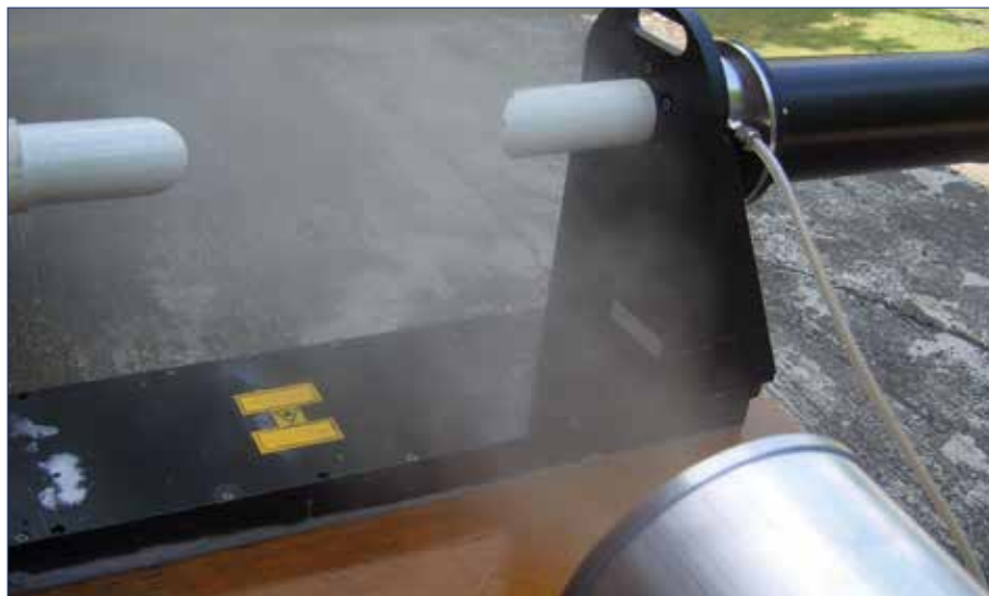
Figure 24. Measuring the spray droplet spectrum of a vehicle-mounted cold fogger
