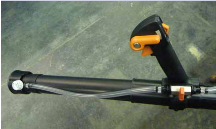
Figure 13b. Showing controls on the lance of a motorized knapsack mistblower
