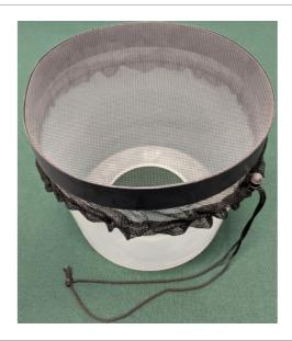
6. Turn the capture chamber over so that the barrier net is on the bottom and place it on top of the bucket.
