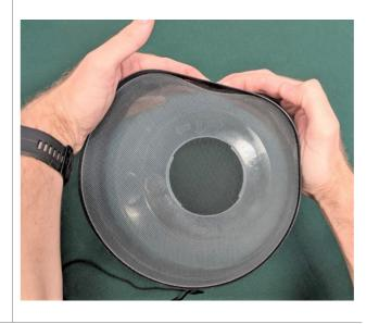
b. Ensure the black ring is evenly placed over the base of the capture chamber.
