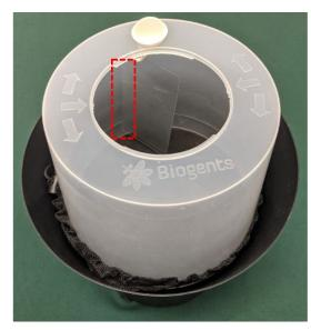
8. Insert the entrance funnel into the top of the capture chamber with the arrow of the entrance funnel pointing to the inward arrow on the capture chamber.
