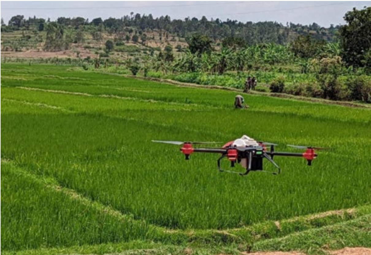
Drone application of larvicide over irrigated agricultural land. © Seth Irish
