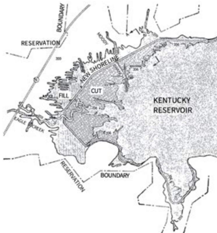
Fig. 7. "Cut and fill" project at Eagle Creek, Kentucky reservoir, Tennessee Valley Authority, 1947
