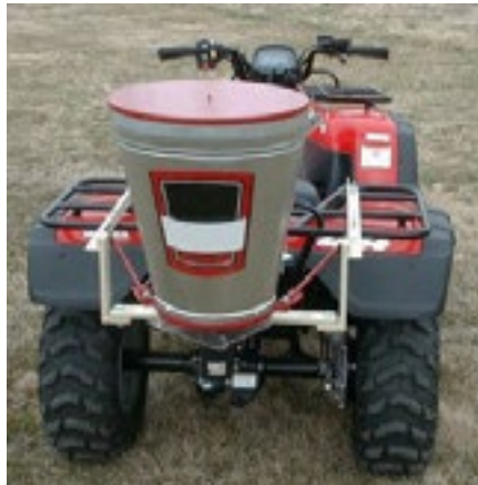
Fig. 33. Example of vehicle-mounted rotary spreader
