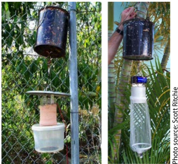
Figure 11: Left: CDC light trap. Right: EVS trap. In both images dry ice (a source of CO 2 ) has been placed into the black tin.
